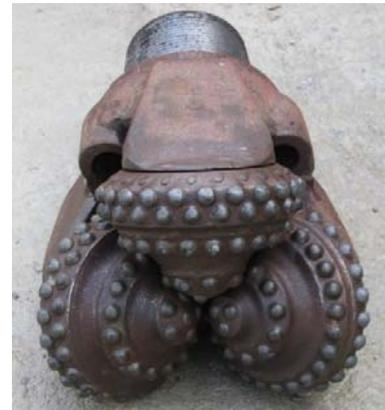
**Fig. 2 Pilot Bit (diameter: 311 mm, weight: 100 Kg).**
