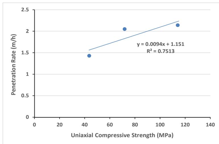
**Fig. 7 Relationship between UCS and penetration rate.**
