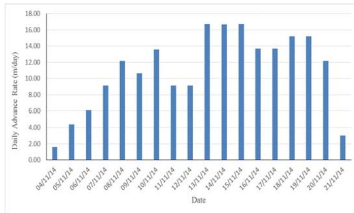
**Fig. 5 Daily advance rate in pilot drilling.**
