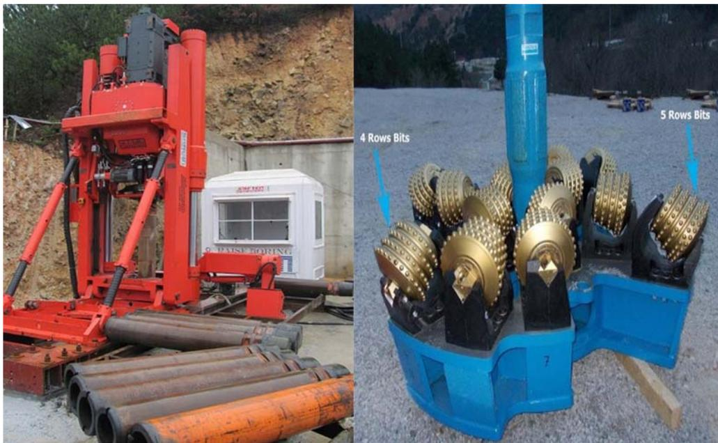
**Fig. 3 The raise bore machine and reaming cutterhead.**
